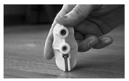
Place the gripper portion of the fixture over the head of the screw.
