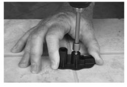
The head of the screw will hit the top of the fixture. The screw will then pull and snap at the score.
