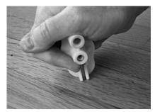
Rock the fixture back and forth until the head of the screw snaps at the score.
