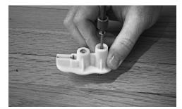
After pre-drilling a 1/8 inch hole down 2 1/4 inches, drive a screw through the taller opening in the fixture.
