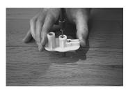
Drive a screw through the shorter opening in the fixture.
