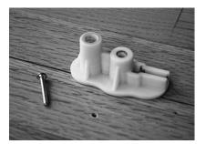
The score is now set 1/5 of an inch below the wood. Fill the hole with putty to finish.
